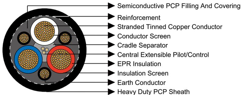
**3×Conductors:** Flexible stranded tinned annealed copper conductor.
